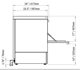
NOTE: Normal operation generates steam that may escape from the door. Materials like wood, laminate etc. are unsuitable for areas exposed to dishwasher steam and only stainless steel surfaces is recommended.
